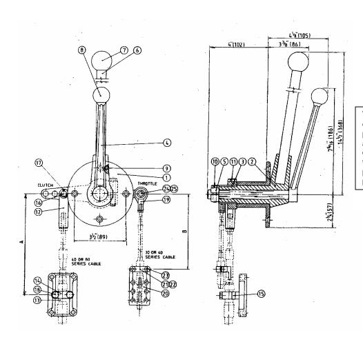
To determine dimension "A", the cable must be in the mid position with the clevis attached. To determine dimension "B", the cable with the rod end attached, must be pushed in for pull governors and pulled out for push governors.
